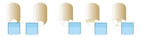
Trimming with trim 90 for FIB, sectioning in the SEM (3View, Volumescope)
