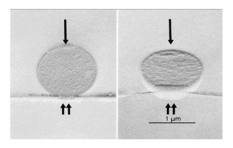
Sectioning of a polystyrene sphere embedded in epoxi resin
