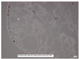
Sample block surface of a spruce needle after sectioning with an ultra 45° knife (above) and an ultra sonic knife (below)
