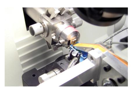
Collecting sections on a tape for imaging in the SEM
