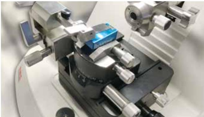
A substrate is clamped to the ASH2 and placed in the water of the knife trough. After sectioning, the water is slowly removed and the section ribbons adhere to the substrate.
