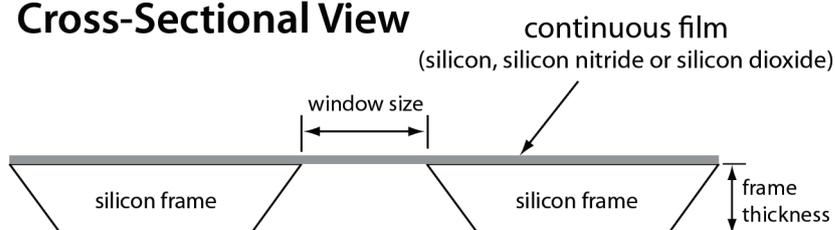
TEM and X-Ray Windows are packaged in silicone gel-boxes with their suspended membrane films facing up (see cross-section). The suspended membrane side of TEM and X-Ray Windows should never be placed onto another surface in the opposite „face-down“ orientation.
