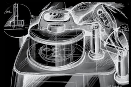
The handle shape is suitable for opening/closing the lid, the angle of the screen is optimized for better digital communication, and the body is adjusted to smooth ampule handling. All details ensure easy operation and maintenance.
