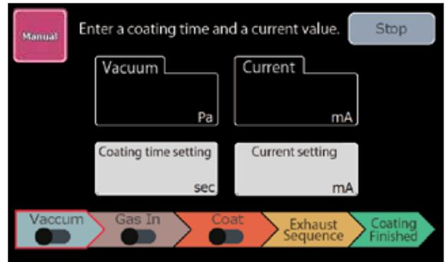
Manual operation option is available. You can set the timing of gas inflow, the coating time and the current value.
