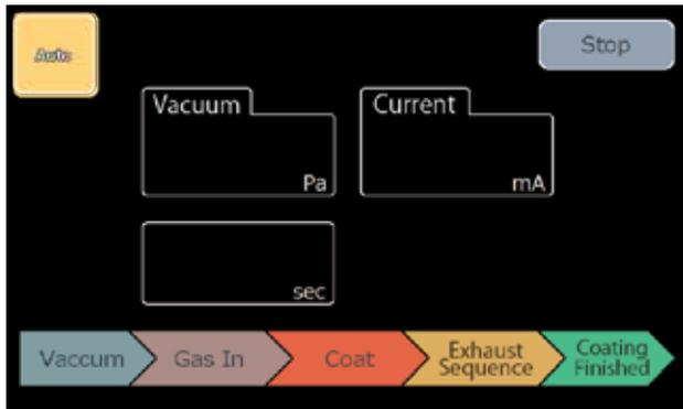
All you have to do is enter a film thickness value. Vacuuming, coating, and exhaust sequence is executed automatically.
