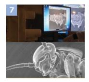
After evacuation, start observation immediately. (NanoSuit (barrier layer) is formed by electron beam irradiation.)
