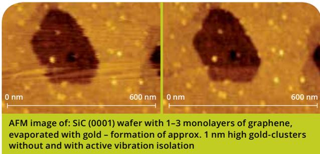
AFM image of: SiC (0001) wafer with 1-3 monolayers of graphene, evaporated with gold – formation of approx. 1 nm high gold-clusters without and with active vibration isolation
