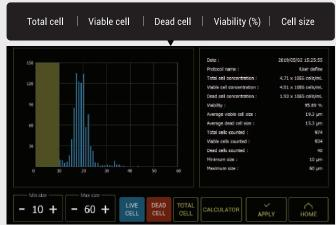
EVE™ PLUS measures the number and concentration of total cells, viable cells, dead cells. It provides viability results and cell size gating.
